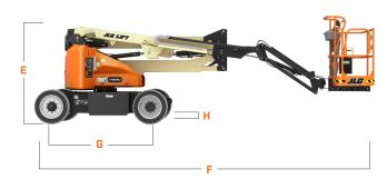
A. Platform Width 30-in / 76-cm B. Platform Length 60-in / 1.52-m C. Machine Width 5-ft 9-in / 1.75-m Tailswing 0-in / 0-cm E. Machine Height 6-ft 7-in / 2.01-m F. Machine Length 21-ft 2-in / 6.45-m G. Wheelbase 6-ft 7-in / 2.01-m H. Ground Clearance 8-in / 20-cm
